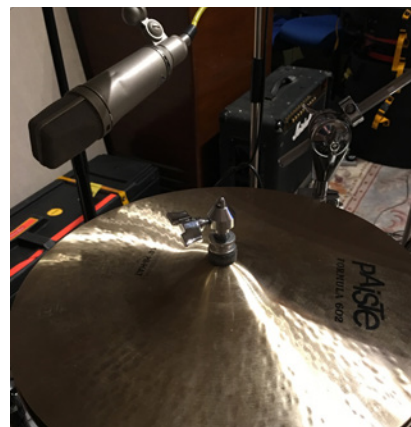
For the hi-hat, a U87 was set to fig-8 mode, and the side nulls were aimed at other cymbals for maximum rejection.
