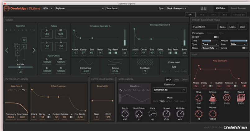
The Digitone Overbridge editor runs standalone or as a plug-in, providing control, sync, total recall and audio inputs to your DAW.
