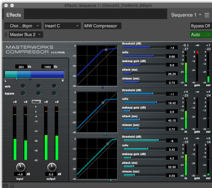
With three user-selectable bands, MW Compressor gives you the ability to apply different amounts of compression to low, mid and high frequencies.
