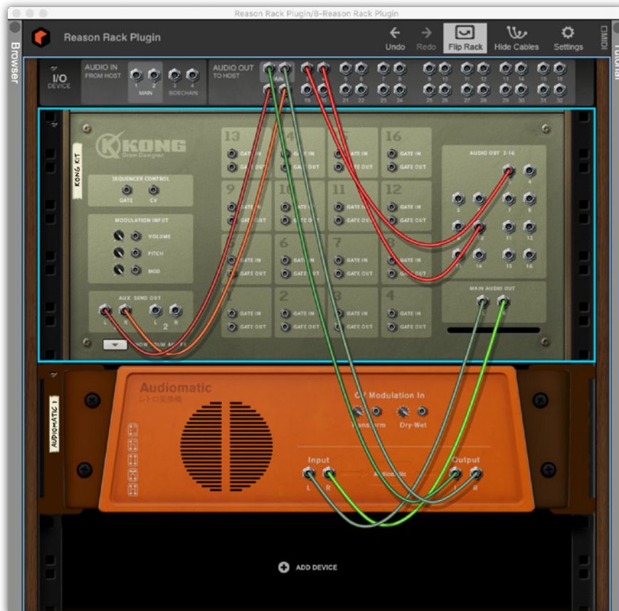
Reason's auto-cabling takes care of most patching for you, but you can flip the Rack plug-in to the rear view and manually patch different input and output busses.
