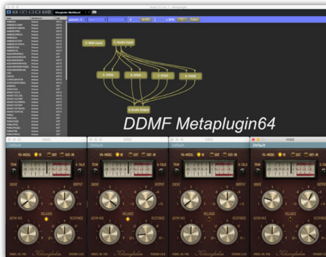
Here, Metaplugin has been used with its bundled multiband splitter to create a four-band saturator, with separate instances of Klanghelm's freeware IVG12 plug-in. When using the splitter, the signal can be recombined by dragging multiple outputs to a single input.
