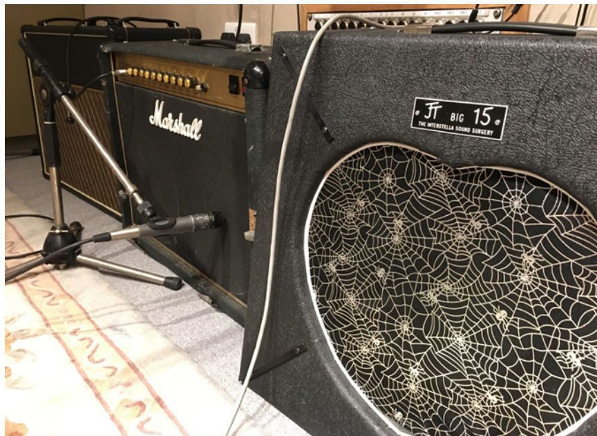
To capture Rossi's guitar sound, a Shure SM57 facing the centre of the cone of a Marshall JCM900 combo made the biggest contribution, but this was mixed with a more distant Neumann KM183 omni room mic set up at head height.
