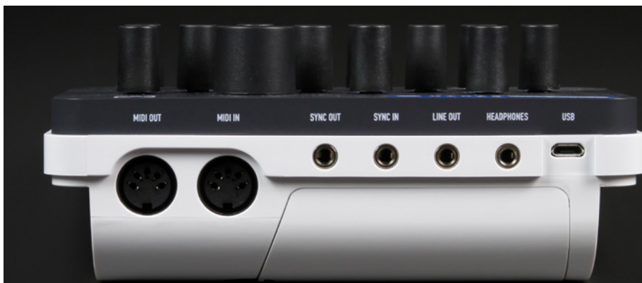
The big news on the Craft Synth 2.0's back panel is the full-size MIDI I/O ports. The accompanying sync I/O, line out and headphone ports are all on mini-jack sockets and there's a mini-USB port for power and computer connectivity.
