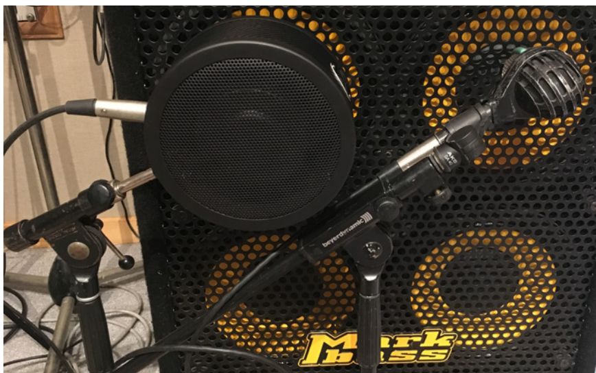
The Markbass cabinet was miked up with an AKG D112 and a Subkick-style Solomon mic, but two DI signals were also captured for maximum flexibility — one direct from the instrument, and one post the Markbass head's preamp stage.
