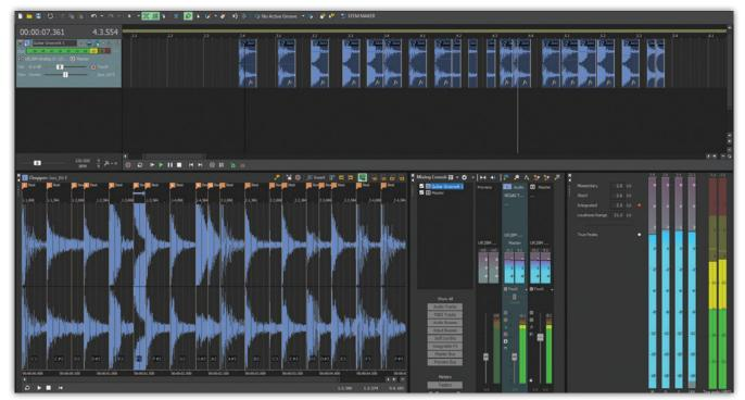
most DAWs have an automatic audio transient-marking process that allows you to creatively process the timing of recorded audio. Sometimes you can even successfully quantise audio just like a MIDI part.
