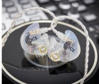
many performers on stage, are not often used in the studio, but high-specification models, like this pair from ACS, are capable of very high quality audio performance, provided they are properly fitted to your ears. This is a custom-moulded set, which is also vented to reduce ear-fatigue and reduce the sense of isolation that fully sealed IEMs can have.
