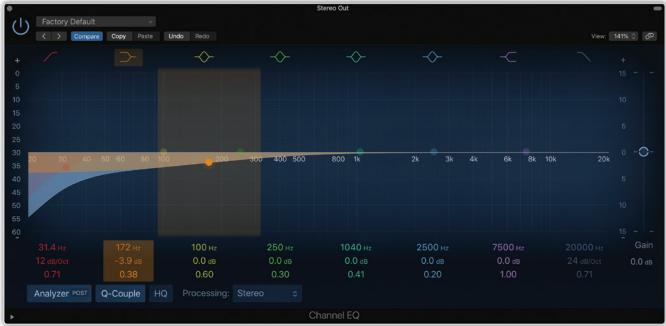
With a lot of sources, there's nothing happening below 100Hz that you'd want to keep in the mix — it'll just be eating up headroom to no audible effect, so you might as well clean it up with a high-pass filter. If you use a very gentle slope, you can even start the roll-off well up into the midrange, without making the sound audibly thinned out — in a lot of sources there is already too much lower-mid energy to combine well with others in a mix.
