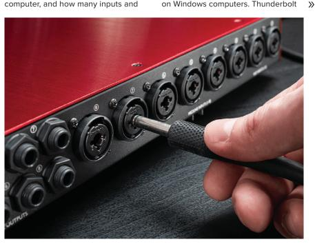
Many interfaces use space-saving 'combi' input sockets that can accept either an XLR cable from a microphone, or a line input on quarter-inch jack.
