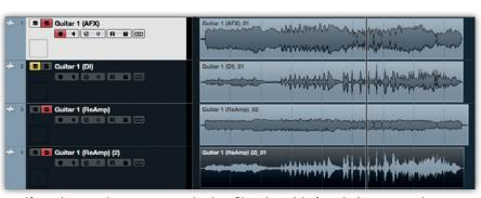
If you always make sure you record a clean DI track straight from the instrument whenever you are tracking guitars, you can experiment with different sounds without having to re-record the part, using re-amping: sending the DI signal to a different amp or processor and re-recording it. You can do this an unlimited number times, until you get the sound you want, or to create layered sounds, as if you had recorded with two or more amps at once.
