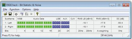
RME's free DIGICheck software tool allows metering, testing, measuring and analysing of digital audio streams, including peak level, RMS level, 'Over' detection, correlation (phase), dynamic range and signal-to-noise ratios, and long-term peak detection.
