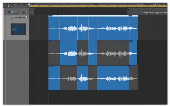
In this simple 'comping' example, the best phrases from two takes have been selected and automatically assembled into the 'comped track' lane above them, with the comping algorithm taking care of any crossfading as necessary. If your DAW doesn't have automatic comping (most now do), you can achieve the same result by assembling the source takes together and cutting out the wanted phrases for assembly on another track.
