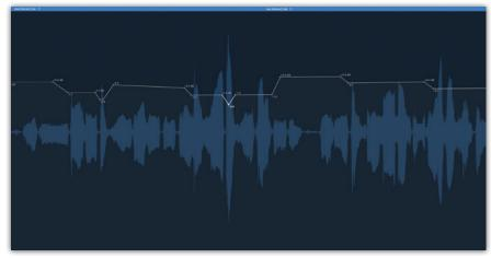
Entering mix-automation vector points manually can actually allow you to be more precise than using a fader or rotary control. Some level adjustments are almost always necessary during the mix, as the song evolves and builds, even if it is only riding vocal level changes and lifting instruments during solos.
