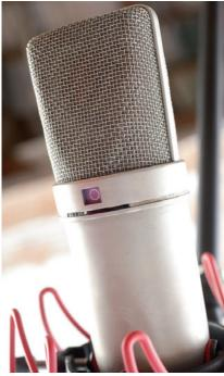
diaphragms, and combining them in different configurations allows the microphone to operate with a cardioid, hypercardioid or omnidirectional pickup pattern. Changing the polar pattern not only affects the amount of room sound or spill from other sources, but also changes the tone of that spill, with the omnidirectional setting pictured here being the most tonally consistent.
