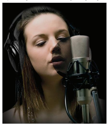
Pop shields successfully dissipate the air blasts that come from pronouncing 'p' and 'b' sounds when singing. You will almost certainly benefit from using one for recording vocals with a capacitor mic. Metal-mesh models may be slightly more transparent to high frequencies than nylon-mesh versions, but either is a good deal better than none.
