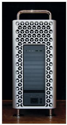
Choosing a tower-format computer allows you to house multiple disk drives, interfaces and co-processor boards neatly within the chassis. Pictured is a latest-generation Mac Pro that will handle any audio-production task you can think of, but it has a price tag to match.
