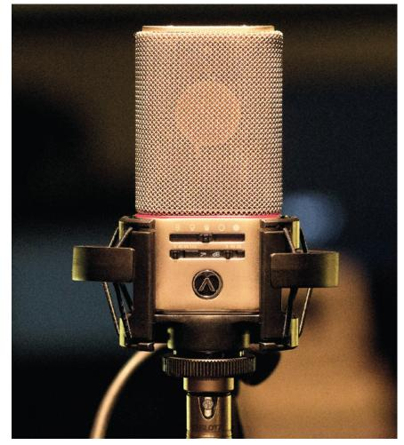
— This sophisticated capacitor model from Austrian Audio offers five pickup patterns, plus pad options and four bass roll-off settings. It also features remote control of the pickup pattern and the ability to take separate outputs from the front and rear of the capsule. If these are recorded separately, they can be combined in different ways during mixing to generate the effect of different pickup patterns being used in the original recording.
