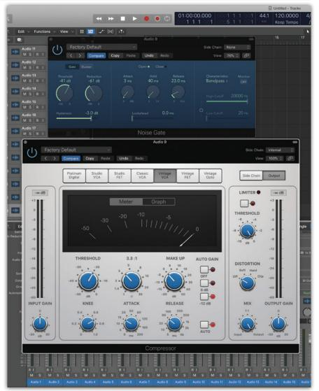
If you need to use a noise gate in a track that also has a compressor patched in, put the noise gate before the compressor to ensure it triggers reliably. If you put the gate after the compressor there will be less of a differential between the levels of the loud sounds and the quiet ones, so the gate will tend to mis-trigger more often.
