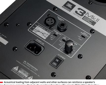
Acoustical loading from adjacent walls and other surfaces can reinforce a speaker's low-frequency response. Most studio monitors therefore offer simple EQ facilities that allow you to adjust the LF response to suit the speaker placement.
