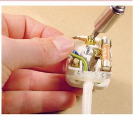
between the primary and secondary windings. Serious problems arise if people decide to break the loop by removing the safety earth in the mains plug instead. This does break the loop, obviously, so any related hum will disappear, but it also means that the equipment is no longer earthed, and any fault that occurs in it is now potentially life-threatening!
