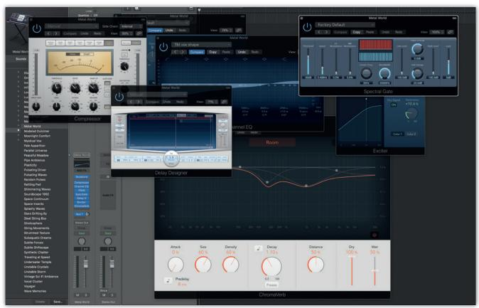
Watch out for software-instrument presets that also install a collection of processing plug-ins, often ending with a reverb. It's not often useful to have a lot of different reverb plug-ins within a mix, and the channel as a whole is usually designed to make the instrument stand out and sound impressive, which may not necessarily be what you want for the track!
