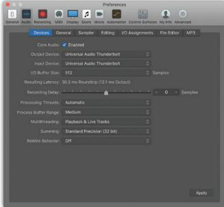
If you've been recording with a small buffer setting to minimise latency, you can switch to a much bigger buffer to ease CPU load and allow more plug-ins when mixing.
