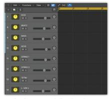
mix bus isn't always the easiest way to structure a complex mix with a large number of sources. Creating logical groups of tracks to be sent to different buses, which then feed on to the mix bus, allows you to control your mix more efficiently using just use the bus faders for the overall balance.
