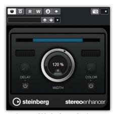
A stereo width plug-in can give the impression of sounds appearing to emanate from beyond the width of your speakers
