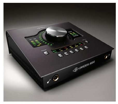
$\blacksquare$  A quarter-inch jack input marked with a guitar symbol, such as this one on a UA Apollo Twin Mkll, usually means that is has a high input impedance, around  $1M\Omega$ , which is about the same as most guitar amps. This ensures that it will work well with conventional passive electric guitar circuitry connected directly, either to achieve a clean DI sound, or to work with guitar-amp modelling software.
