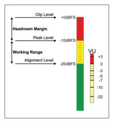
To achieve the same amount of headroom in a digital system as working to 0dB on an analogue VU meter, you'd have to target around -20dBFS.
