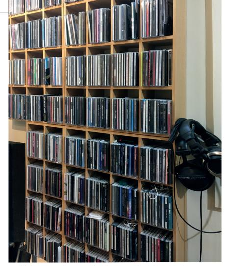
Diffusion and scattering are your friends here, best achieved with the help of uneven reflective surfaces, such as loaded shelves, CD racks, spare equipment and so on.
