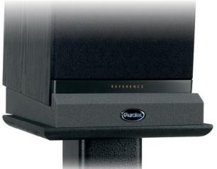
If you need to stand your monitors on a shelf or desk, a well-designed decoupling system like this one from IsoAcoustics can be effective at preventing low-frequency vibrations being transmitted into the desk. In some instances, the improvement can be surprisingly noticeable. Foam decouplers, such as this Auralex MoPad, which act as both a spring and a damper, can also help to prevent some vibration from being transmitted from a speaker to your studio furniture.
