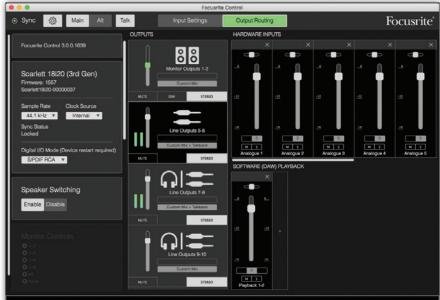
a round-trip latency of under 5ms can be hard to achieve, especially on USB interfaces. For this reason, many audio interfaces have a built-in mixer that allows us to hear input signals without waiting for them to pass through the computer and recording software — a feature usually called 'Direct Monitoring'. On some small 'desktop' interfaces, this mixer is controlled using a simple knob that adjusts a balance between input signal and playback from your
