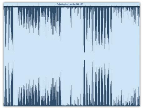
A heavily clipped audio waveform is instantly recognisable, with large flat-topped areas, but short-term clipping is much harder to detect visually.
