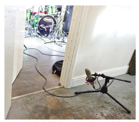
An unusual mic position, blended in with more conventional miking can give a familiar sound a unique extra quality. Record it to its own track so you can experiment with compression and EQ in the mix. If you haven't got a big enough space to make 'room' mics work, placing one just outside can still work well to achieve the same effect. And if it is outside the room, it might as well be mono.
