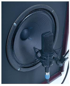
A loudspeaker is really just like an acoustic instrument, in that the sound does actually vary at different points across its surface. It may be 'traditional' to mic speakers really close like this, but there is often a more complete, integrated sound to be had slightly further away, and aiming somewhere between the centre and edge of the cone.
