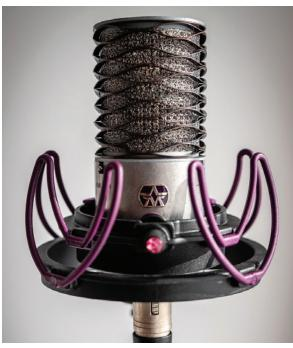
'end-address' capacitor cardioid you can see vent slots in the housing. These are the entrance to the acoustic labyrinth behind the diaphragm through which it achieves its directionality.
