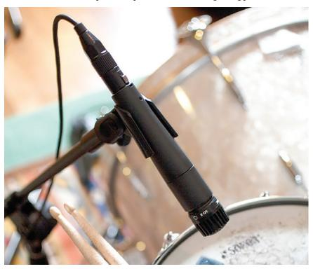
The venerable Shure SM57 remains a great 'all-rounder', equally at home on snare drum or a guitar speaker. It has a strong midrange without too much of a presence peak, making it useful for a wider range of sources than the vocal-optimised SM58. Try it on acoustic guitar for a more robust rhythm part than a capacitor mic would give you.
