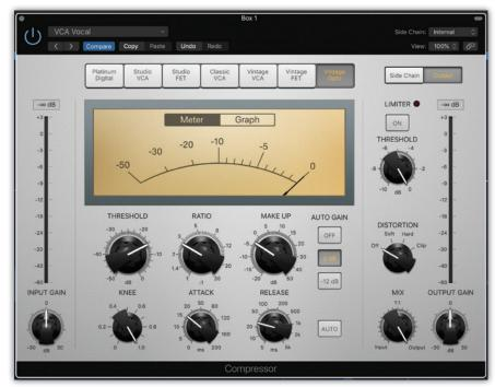
— Treat dynamics presets as a starting point — they'll probably have sensible Attack and Release settings — but always be prepared to adjust Threshold and Ratio.
