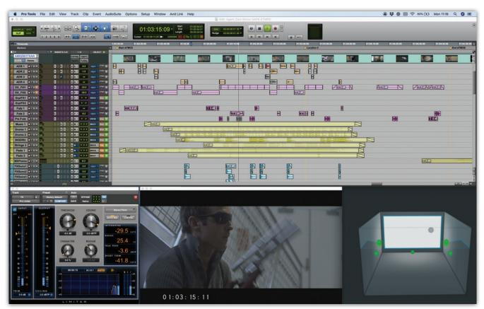
wid's Pro Tools DAW differs slightly from the common working paradigm in that the main screen used for the arrangement of clips/regions is also the edit screen, as you can zoom in to sample level. Most other DAWs use a dedicated edit window for deep-level audio editing.
