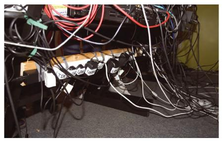
A lot of home studio equipment is now powered from an external power adaptor rather than a direct mains connection. It is well worth labelling adaptors with the name of the unit they supply, as you can easily find you have a few of them, all looking the same but supplying different voltages. Some units are protected against an over-voltage input, but by no means all. By the time you see smoke, it is usually too late!
