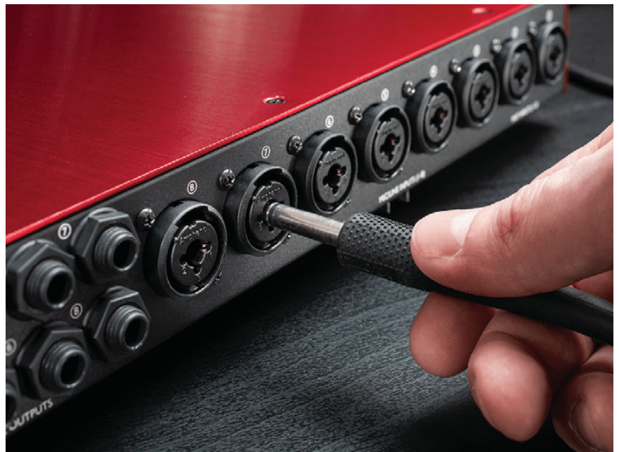
■ Many interfaces use space-saving 'combi' input sockets that can accept either an XLR cable from a microphone, or a line input on quarter-inch jack.
