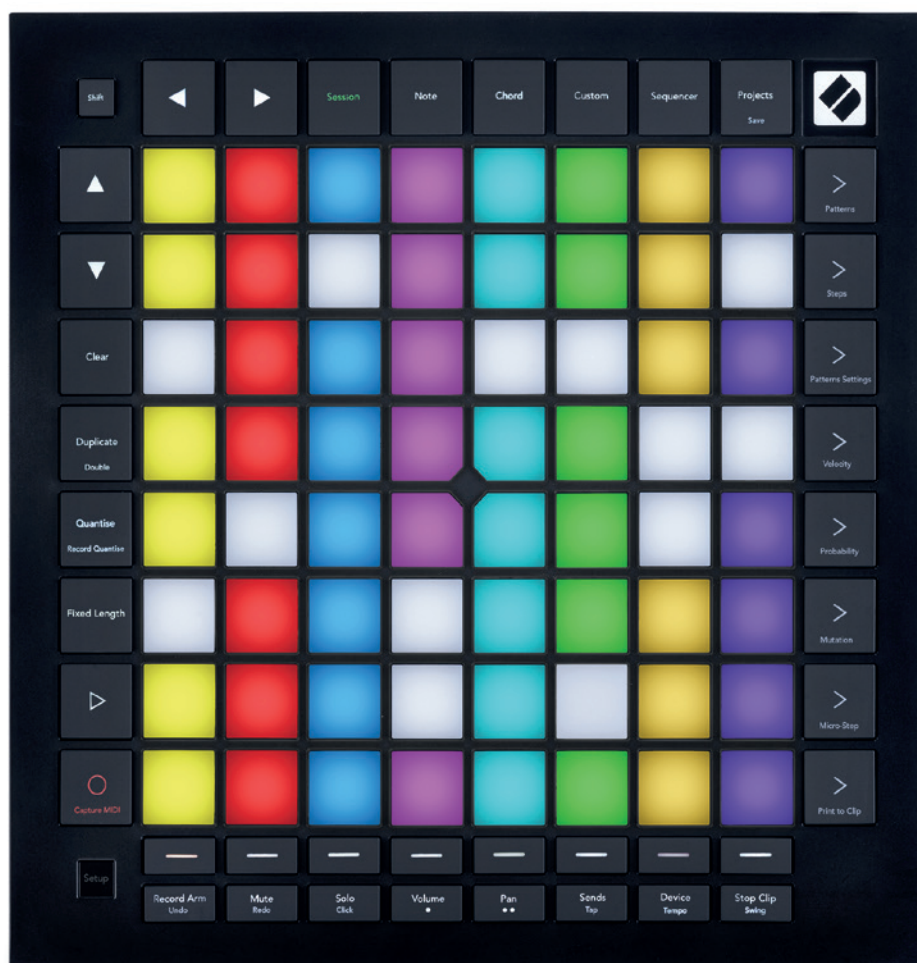
Novation's Launchpad controller hardware is an ideal partner for the loop and sample-based operation of Ableton Live, with 64 velocity- and pressure-sensitive RGB pads that mirror the software's on-screen layout.
